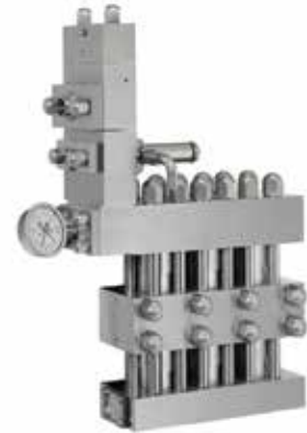
RANNIE THREE-PIECE CYLINDER BLOCK WITH HYDRAULIC ACTUATION
